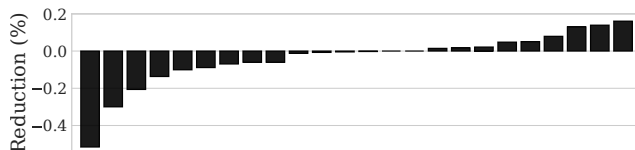
Figure 19. A breakdown of SalSSA[t = 1] on the djpeg benchmark. The actual contribution to the final code size for each merge operation deemed profitable by the cost model.
